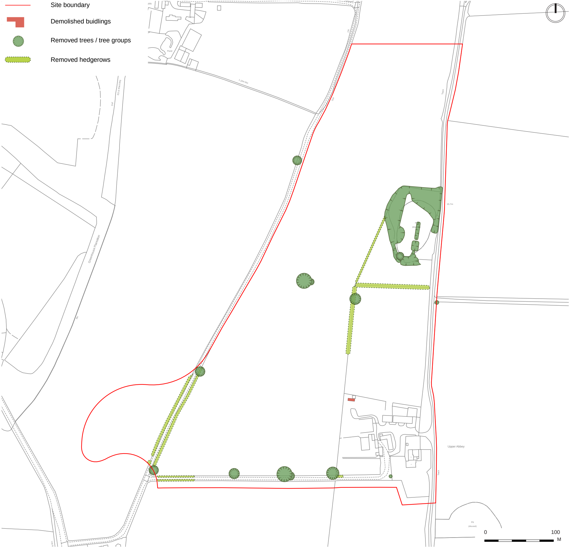
Figure A.57: Clearance and Demolition Plan
