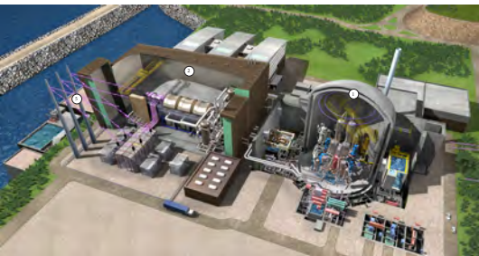
Illustrative UK EPR™ Nuclear Reactor and Turbine Hall layout
