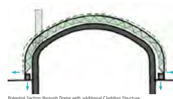
Potential Section through Dome with additional Cladding Structure
